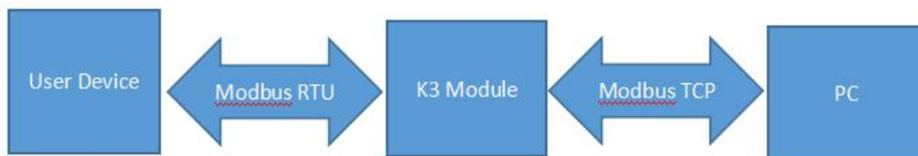
Diagram 6-2 function description for ModbusTCP to modbus RTU
